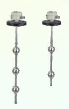
A magnetic float moves up and down on probe immersed in a liquid. The float energizes the hermitically sealed sensors, which change from NO to NC otherwise as the float-passes them.
